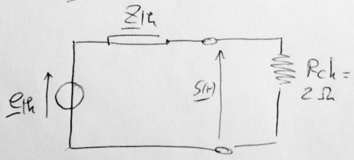
$$\underline{S}(t) = \underline{e}_{Rt} \times \frac{R_{ch}}{\underline{Z}_{Rt} + R_{ch}}$$
