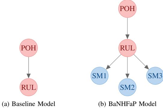
Fig. 2: Comparison between the baseline and proposed prediction models for HDD failures based on SMART features.
