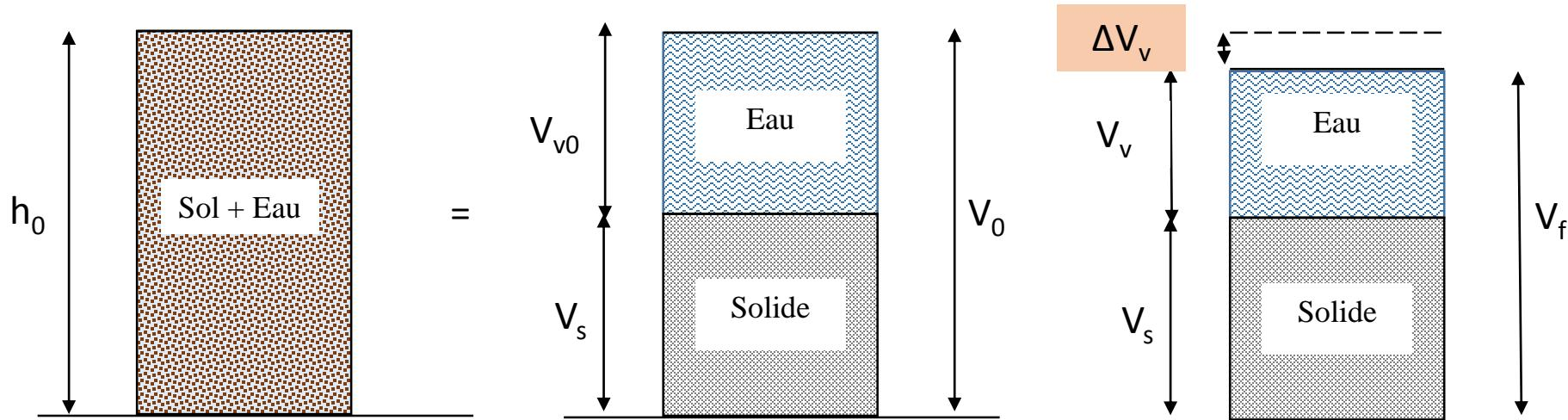
$$\frac{\Delta h}{h_0} = \frac{\Delta V}{V_0} = \frac{\Delta V_v}{V_0} = \frac{\Delta V_v}{V_s + V_{v0}} = \frac{\Delta e}{1 + e_0}$$
